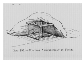
Fig.195. - Heating arrangement in floor. 図195. 掘り炬燵
