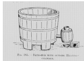
Fig.183. - Bath-tub with outside heating-chamber.
