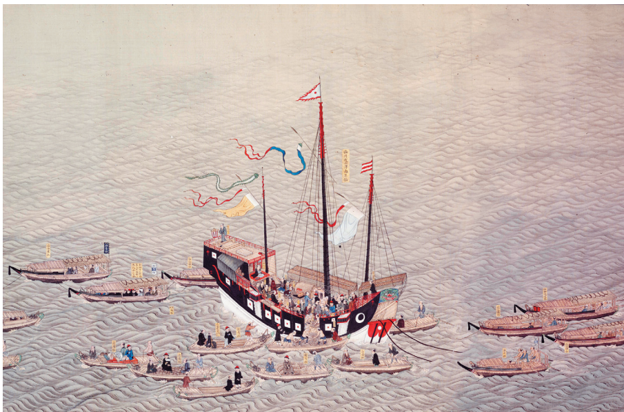
Figure 1. Chinese vessel unloading into flat-bottomed boats ( sampan ). Vessels were moored in the open bay close to shore; speedy unloading was important to admit replacement of the cargo with ballast to stabilize vessels in what were at times stormy waters. (Courtesy of Nagasaki Museum of History and Culture.)
