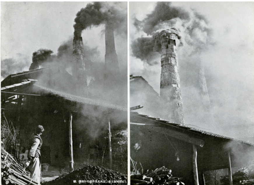
Figure 4. Tōmatsu Shōmei, Asa, entotsu kara hono'o ga miereba, ato sūjikan da (If flames can still be seen coming out of the chimneys in the morning, the firing will go on a few more hours), 1955. In Iwanami 1955, pp. 32–33.
